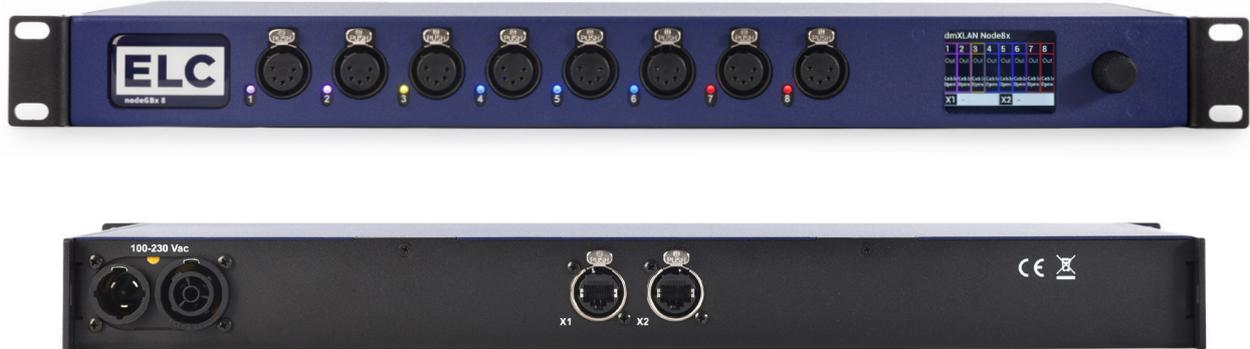
The dmXLAN node8GBx DMX / Ethernet Node comes with an integrated dual GBit ports and colour touch-sensitive display. It offers 8 bidirectional 5-pin XLR female connectors (optically isolated) on the front panel, which can be used as DMX outputs, DMX inputs or DMX outputs with RDM. The two Gigabit Ethernet ports are located on the rear of the unit.
