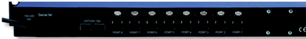
Looking from the back the most left slot is for port 7 and the right option slot (next to port 8) is used for port 8.
